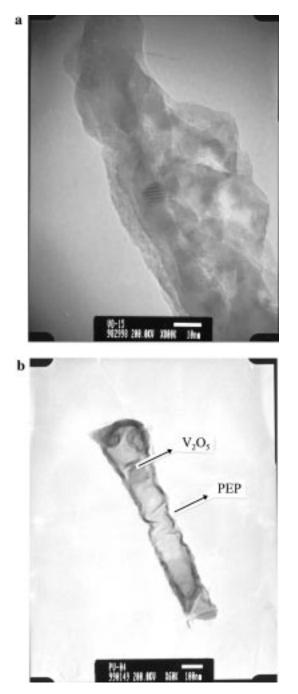
Figure 5. TEM of  $PEP/V_2O_5$  composites (30 wt %:70 wt %): (a) high magnification; (b) low magnification.
