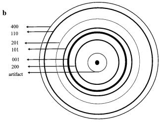
**Figure 6.** Electron diffraction pattern of  $V_2O_5$  from TEM: (a) original diffraction pattern; (b) schematic diffraction pattern and the assignments of indexes.
