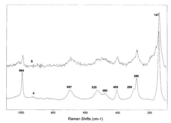
Figure 3. Raman spectra of (a)  $V_2O_5$  (No. 5); (b) PEP/ $V_2O_5$  (5 wt %:95 wt %).
