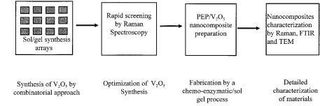
Figure 1. Schematic of the combinatorial process to synthesize PEP/V<sub>2</sub>O<sub>5</sub> nanocomposites.
