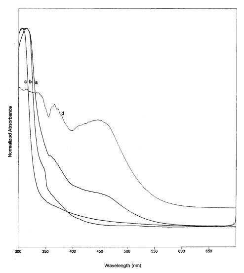
Figure 7. UV-vis spectra of samples in THF: (a) PEP/V<sub>2</sub>O<sub>5</sub> (30 wt %:70 wt %); (b) PEP/V<sub>2</sub>O<sub>5</sub> (5 wt %:95 wt %); (c) PEP; (d) V<sub>2</sub>O<sub>5</sub>.
